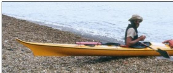
*The HM Nordkapp stern, showing the keel line extended to almost under the stern horn
