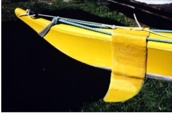
*The skeg in position when paddling; the shock cord stretched tight to the stern horn of the kayak*
