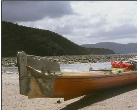
*The blade in its retracted position on deck*
