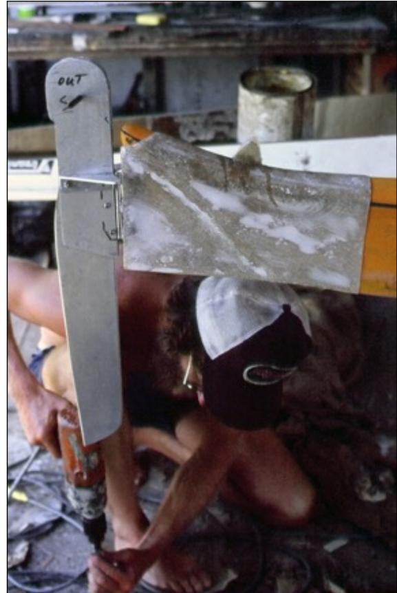
*Construction of the aluminium over stern rudder assembly at Tony Turbett's workshop in Brisbane. The rudder is attached by a stainless steel hinge glassed into a fibreglass 'shoe or sleeve' that allowed the stern horn of the Nordkapp to remain intact – but I could remove the whole lot if I didn't like the rudder!*
