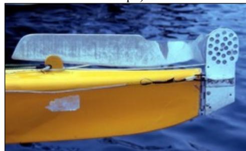
*The overstern rudder mounted on Hiya Kaze – the kayak used for the 4,021 mile paddle around Japan. The holes were to reduce weight*
