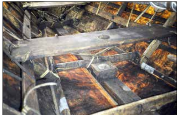
Sunlight glows through the translucent walrus skin, The mast step for sailing visible with hole in the seat to support the mast for sailing
