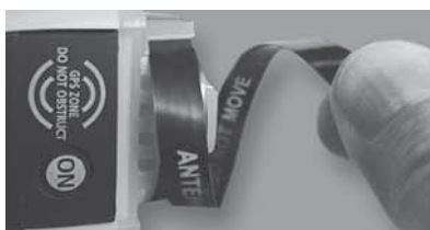
Two photos showing the coiled position of the antenna (left) and unfurled or in an erect position.
